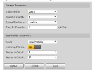
Figure 2-20 Snapshot settings-loop mode
