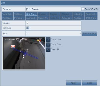
Figure 9. 6 Draw Line for Line Crossing Detection
