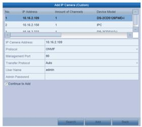
Figure 2. 20 Custom Adding IP Camera Interface
