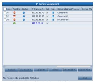
Figure 2. 18 Adding IP Camera Interface
