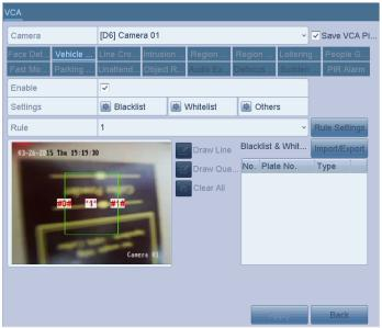
Figure 9. 3 Set Vehicle Detection
