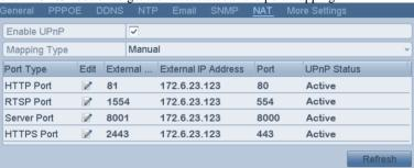
Figure 11. 17 UPnP<sup>TM</sup> Settings Finished-Manual
