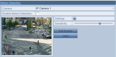
Figure 5. 12 Motion Detection
