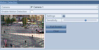
Figure 8. 2 Set Detection Area and Sensitivity
