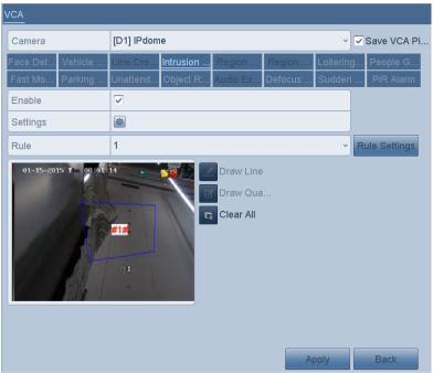
Figure 9. 8 Draw Area for Intrusion Detection
